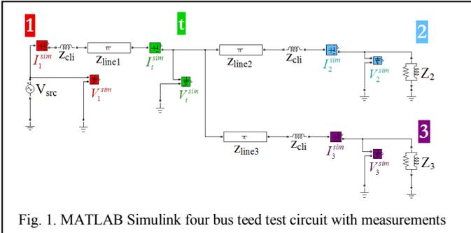
Fig. 1. MATLAB Simulink four bus teed test circuit with measurements
